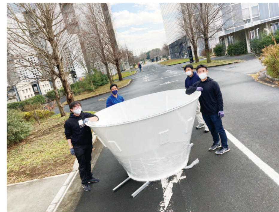
Fig. 2: The forebaffle for the Simons Observatory Small Aperture Telescope carried by the IPMU CMB group member.
