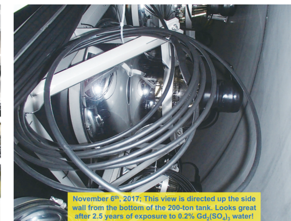
Figure 3 : Looking up the side wall of the empty EGADS tank after 2.5 years of soaking in Gd
