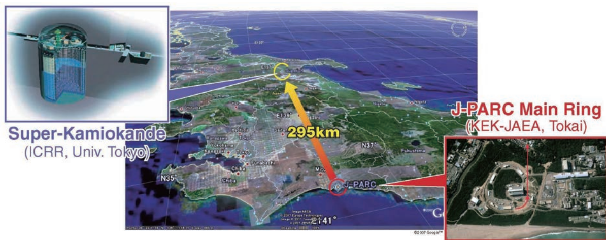
Fig. 1: The T2K experiment produces a beam of muon (anti) neutrinos at the J-PARC accelerator and detects neutrinos after oscillations at Super-Kamiokande, 295 km away.
